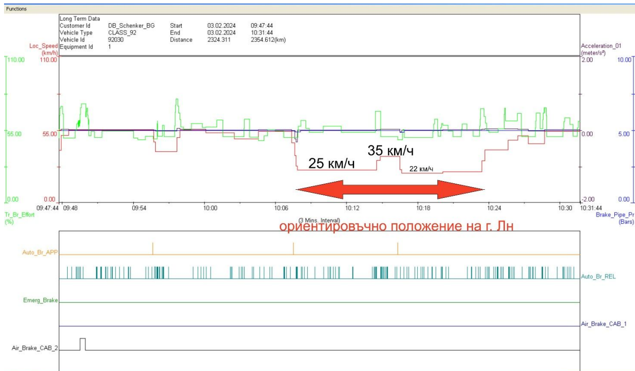
Fig. 2.13. Decoding of the record for movement of locomotive № 91521688030-1 in the period from 09:47 a.m. to 10:31 a.m. on 03.02.2024 along the section between Simeonovgrad station to Radnevo station with focus on the passing through Lyubenovo transmission station
