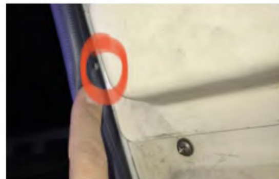
Correct installation: Inflation hole facing the inner side of the door
